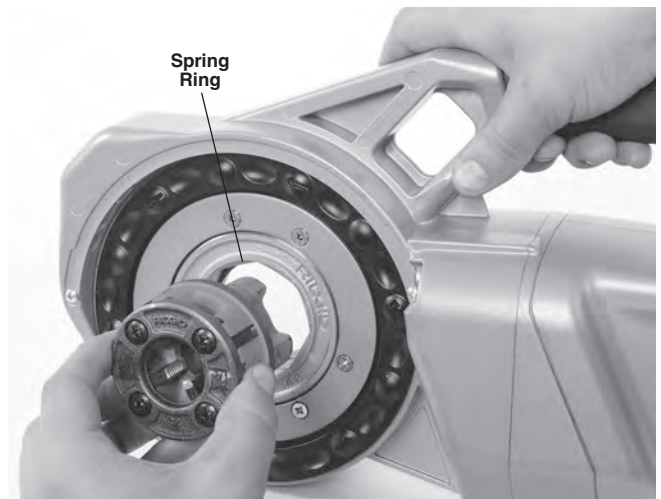
Figure 8 – Installing 1 \frac{1}{4} " or Smaller 11-R Die Heads (760 FXP 11-R only)
